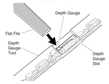
Figure 22 - Depth Gauge Tool On Chain
